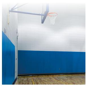
Covers are made of highly tear resistant vinyls available in a range of standard and custom colours. Most pads can also be supplied with wood backing. Foam cores are made of cross-linked polyethylene and polyurethane and they are available in various thicknesses and densities, depending on individual needs. Enhance your interior walls with safety and sound proofing
