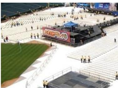
**Terraflor** protects turf at Stadiums and Sports Arenas when the playing area is used for non-sporting events. Designed to protect the turf at Stadiums and Sports Arena's when the playing area is being used for non-sporting events. It allows the passage of air and light and creates a moist atmosphere under the tile, without build-up of heat. These are the essential elements for keeping grass healthy and green.
